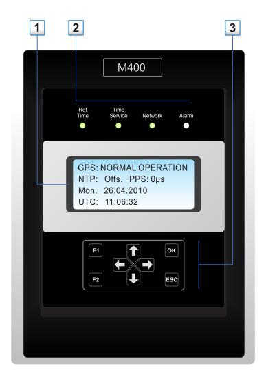
1. The main menu is displayed after switching on the device and having completed the initialization phase. In the main menu the most important status information are displayed. In the top line of the display the operating mode of the reference clock / reference time is shown. Instead of "GPS: NORMAL OPERATION" the messages, "GPS: COLD BOOT", "GPS: WARM BOOT" or "GPS: UPDATE ALMANAC" can appear. In case the antenna connection is interrupted, the following message is shown: "GPS: ANTENNA FAULTY".
